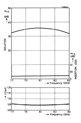
Typical performance as a function of frequency at a working temperature of 20  $^{\rm o}{\rm C}_{\:\raisebox{1pt}{\text{\circle*{1.5}}}}$
