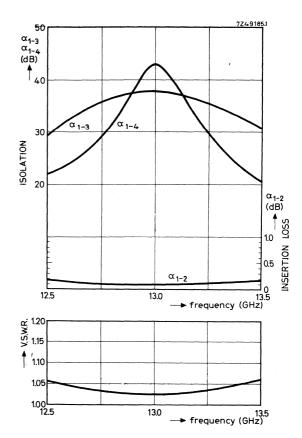
Typical performance as a function of frequency at a working temperature of 20  $^{\circ}$ C.
