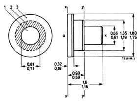
Compression force on mounting surfaces x-x and y-y: max. 2.45  $\ensuremath{N}$
