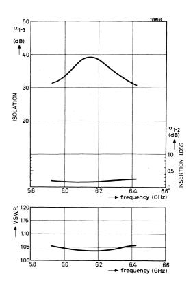
Typical performance as a function of frequency at a working temperature of 20  $^{\rm o}\text{C.}$
