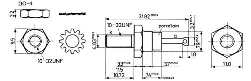
Diameter of hole in heatsink: max. 5.2 mm Accessories available: 56295 (56262A)
