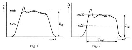
The current pulse must be substantially square and the ripple over the top portion of the current pulse must be kept as small as possible to avoid unwanted frequency modulation due to pushing effects. The spike on the top portion of the pulse must be small to avoid excessive peak pulse current. The leading edge of the pulse must be free from irregularities.
