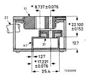
Fig. 1 Cross section of the mount (coupler)
