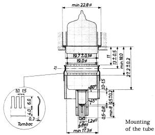
$<sup>\</sup>frac{1}{2}$ ) In order to make good contact these sockets should be slotted.  $\frac{1}{2}$ ) Line of contact.
