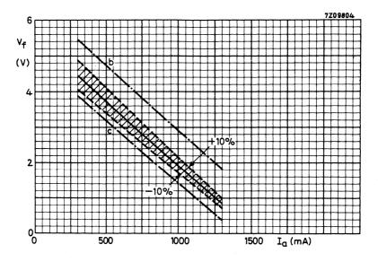
Filament voltage reduction curve.
