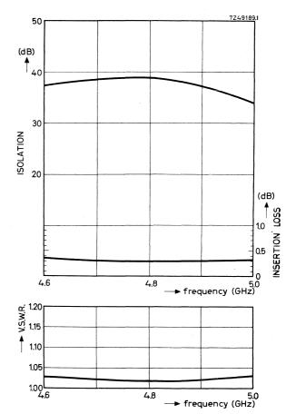
Typical performance as a function of frequency at a working temperature 20 °C.
