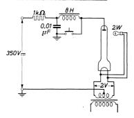
The minimum value of  $V_{ign}$  is only valid if some ambient illumination is present. Hence in darkness the presence of a small light-source (about 2 W) is necessary.
