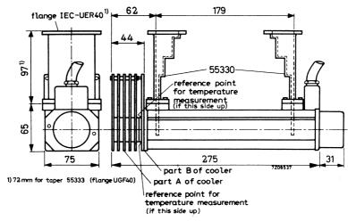
Mount 55329 with convection cooling and waveguide tapers 55330.
