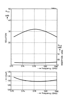
Typical performance as a function of frequency at a working temperature of 20 oC.
