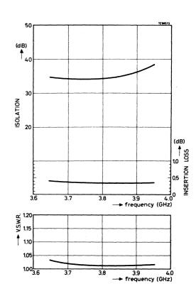
Typical performance as a function of frequency at a working temperature of  $20\ ^{\circ}\text{C}$ .
