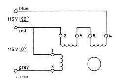
Two-phase, 400 Hz supply 90° shift between phases
