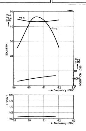
Typical performance as a function of frequency at a working temperature of 20  $^{\circ}\text{C}_{\:\raisebox{1pt}{\text{\circle*{1.5}}}}$
