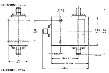
Frequency range Isolation Insertion loss V.S.W.R. Maximum power (c.w.) Temperature range
