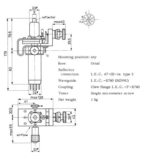
The tube is equipped with the output waveguide I.E.C.-R740 (RG99U) with claw flange I.E.C.-F-R740 and clamping ring. A loose claw flange is added for adaptation to other coupling systems if necessary.
