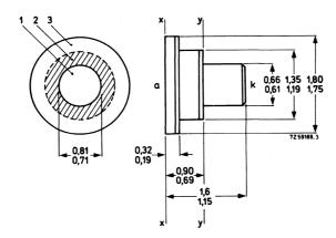
Compression force on mounting surfaces x-x and y-y: max. 2.45 N
