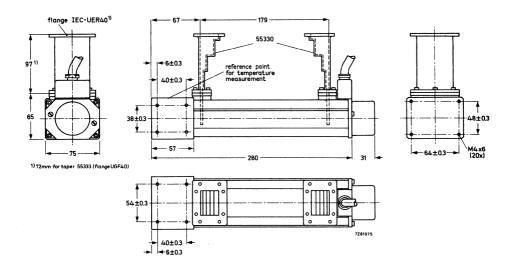
Mount 55332 with conduction (heatsink) cooling and waveguide tapers 55330
