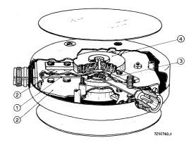
Construction of a coaxial circulator Fig.8
