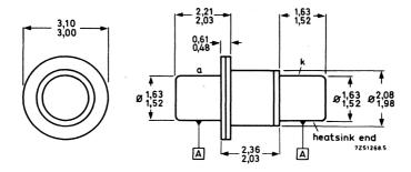
A = concentricity tolerance =  $\pm 0.13$ Type marking on the container The heat should be transferred via the flangeless pin
