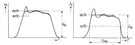
The rate of rise of anode voltage  $(\frac{\Delta V}{\Delta T_{r_V}})$  is defined by the steepest tangent to the
