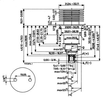
$\underline{\underline{\text{Mounting:}}}$  where possible, the tube should be mounted in the coaxial resonators with the aid of adequately resilient spring contacts.
