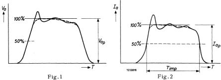
The current pulse must be substantially square and the ripple over the top portion of the current pulse must be kept as small as possible to avoid unwanted frequency modulation due to pushing effects. The spike on the top portion of the pulse must be small to avoid excessive peak pulse current. The leading edge of the pulse must be free from irregularities.
