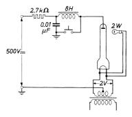
The minimum value if  $V_{\mbox{ign}}$  is only valid if some ambient illumination is present. Hence in darkness the presence of a small light-source (about 2W) is necessary.
