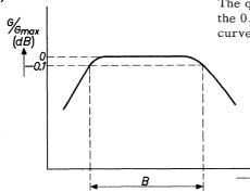
The quoted value is the bandwidth between the  $0.1\,\mathrm{dB}$  points of the flattened response curve.
