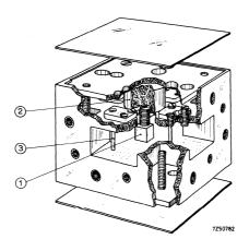
Construction of a waveguide circulator Fig.7
