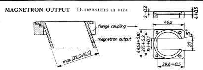
The magnetron output has been designed for coupling to the standard rectangular waveguide RG-51/U by means of a special flange coupling which fits the magnetron to the standard choke flange type UG-52A/U.
