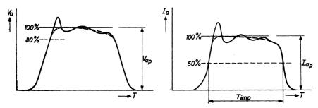
The current pulse must be substantially square and the ripple over the top portion of the current pulse must be kept as small as possible to avoid unwanted frequency modulation due to pushing effects. The spike on the top portion of the pulse must be small to avoid excessive peak pulse current. The leading edge of the pulse must be free from irregularities.
