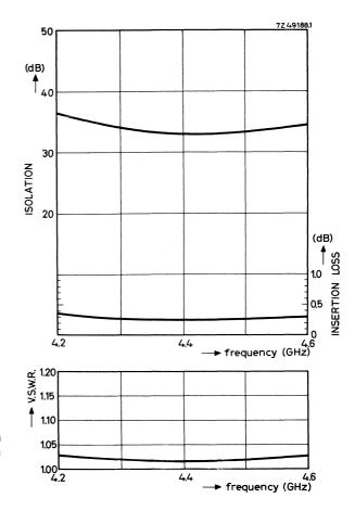
Typical performance as a function of frequency at a working temperature of 20 °C.
