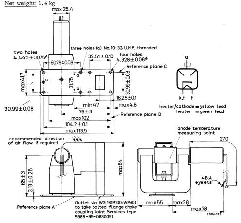
Output coupler: The output connection of the magnetron should be connected directly to a waveguide choke flange type UG-40B/U (5985-99-083-0051).
