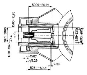
The dimensioned cylindrical surfaces shall be concentric within 0.076 mm
