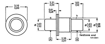
A = concentricity tolerance =  $\pm 0.13$ Type marking on container The heat should be transferred via the cathode pin
