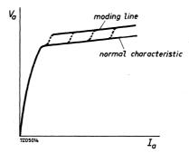
X—Y display of magnetron characteristic (unfiltered supply)
