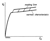
X—Y display of magnetron characteristic (unfiltered supply)
