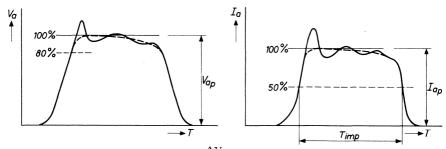
The rate of rise of anode voltage  $(\frac{\Delta V}{\Delta T_{rV}})$  is defined by the steepest tangent to the leading edge of the voltage pulse above 80% of the smooth peak value. Any capacitance used in a removable viewing system shall not exceed 6 pF. For calculation of the rate of rise of anode voltage the smooth peak value must be taken as 12.5 kV.
