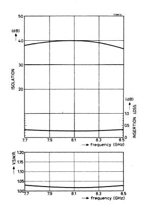
Typical performance as a function of frequency at a working temperature of  $^{\circ}$ C.
