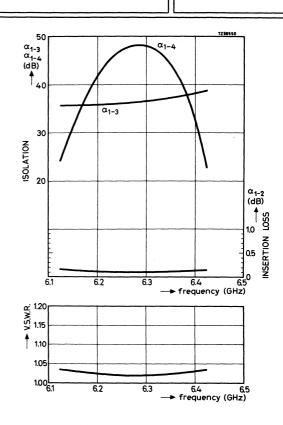
Typical performance as a function of frequency at a working temperature of 20  $^{\rm o}\text{C}_{\:\raisebox{1pt}{\text{\circle*{1.5}}}}$
