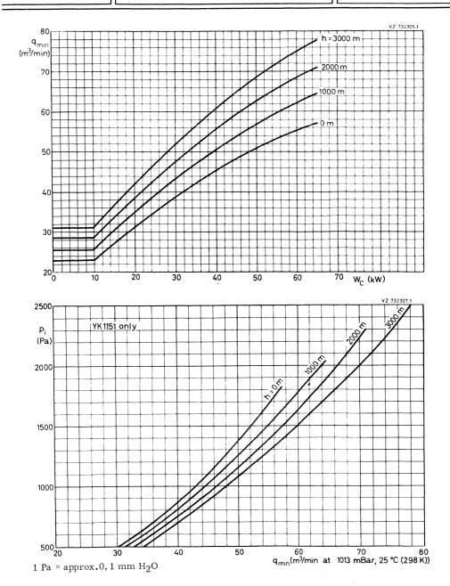
The above curves apply to air inlet temperatures up to 45  $^{\rm 0}{\rm C}\text{.}$
