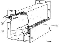
Field displacement type of isolator
