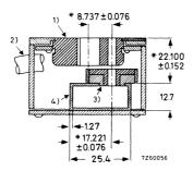
Fig. 1 Cross section of the mount (coupler)
