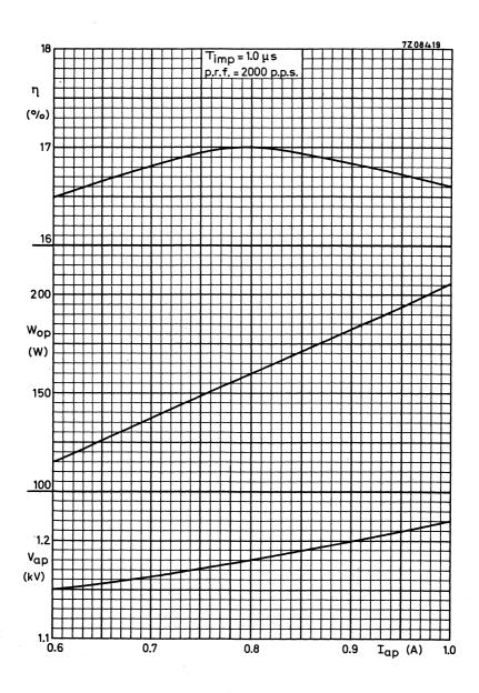
Light-weight packaged magnetron for pulsed service at high altitudes. The tube operates at a fixed frequency within the range 9.345 to 9.405 GHz and the peak output power is 20 kW.
