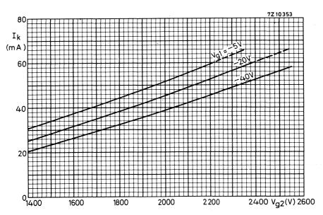
Cathode current = f (accelerator voltage)
