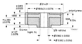
Fig. 3 Top-view of the mount
