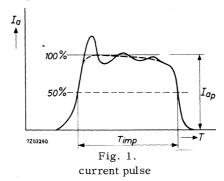
The smooth peak is the max. value of a smooth curve through the average of the fluctuation over the top portion of the pulse.
