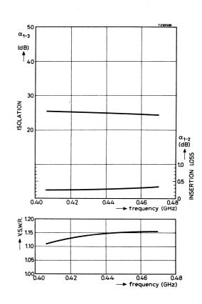
Typical performance as a function of frequency at a working temperature of  $20\ ^{O}\text{C}$ .
