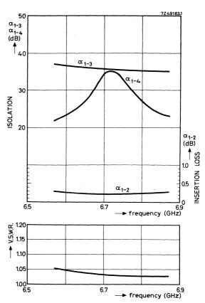
Typical performance as a function of frequency at a working temperature of 20  $^{\circ}$ C.
