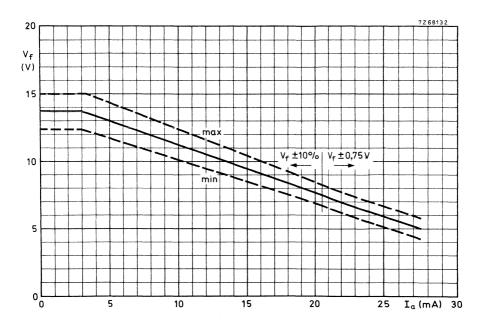
Heater voltage reduction curve
