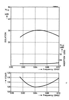
Typical performance as a function of frequency at a working temperature of  $20\ ^{\circ}\text{C}$ .
